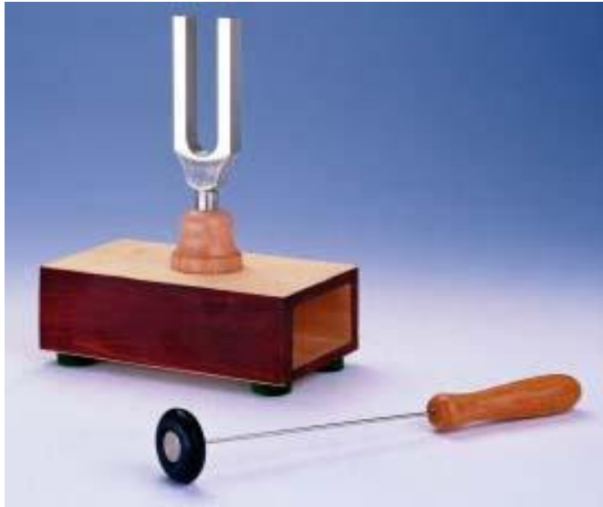
Figure 1.08. Tuning fork with wooden resonator, for the amplification of its sound.
