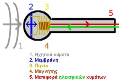
Figure 2.09. How a microphone works.
