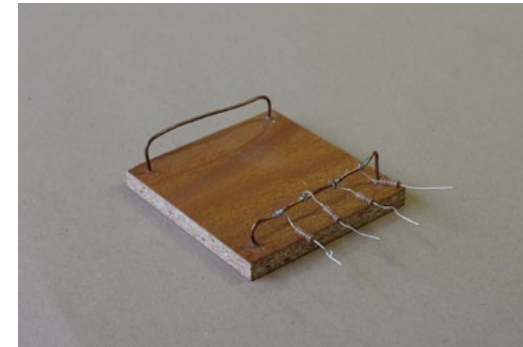
Figure 6.02 DIY mixer for four instruments.
