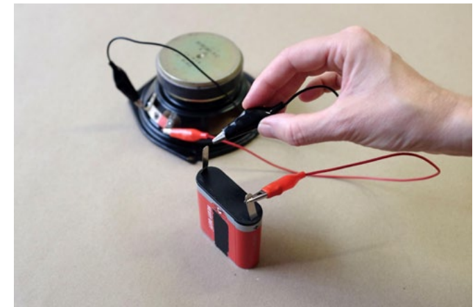
Figure 2.06. Speaker and battery.
