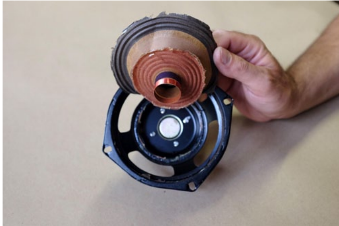
Figure 2.14. A deconstructed loudspeaker. Its shiny orange coil is now visible.
