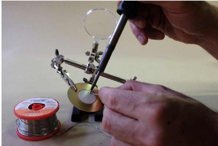
Figure 4.15. Second piezo soldering.
