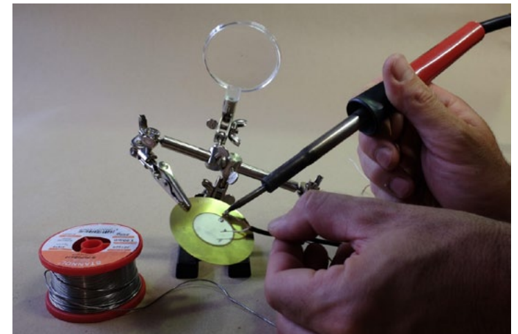
Figure 4.14. First piezo soldering.
