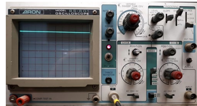
Figure 2.11. Visualising a constant current on an oscilloscope.
