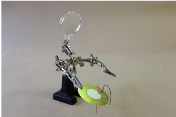
Figure 4.12. Soldering helping hands with piezoelectric buzzer.
